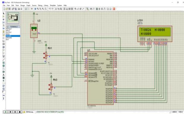
Fig 4 Simulation of Cattle Health Monitoring System in Proteus
